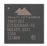
Available in a low cost 11x11mm BGA package and typical power consumption of less than 1W, the TN4010 offers the lowest power and cost MAC solution for next generation NIC and LOM for PC's, Servers and NAS systems, that seek to service the increasing demand of higher network bandwidth, while maintaining backward compatibility with existing Ethernet infrastructure.
