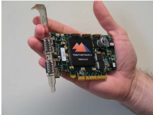
Figure 3 – Tehuti Networks 10 GbE host hardware offload controllers, shown here mounted on a network interface card, reduce latency by optimizing the system’s ability to process packets
